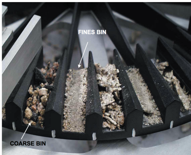
Figure 3. Crushed materials that are smaller than the smallest gap between the plate and the wedge fall into the sorter, which separates the materials into two size categories. The mechanical screening and vibrating process separates large fragments from fine particles causing them to fall into adjacent bins. Once either of the bins have reached peak capacity (coarse or fines, whichever is first), the sample-handling system autonomously shuts off the crusher and moves the sample wheel, placing an empty coarse bin and an empty fines bin under the sorter.
