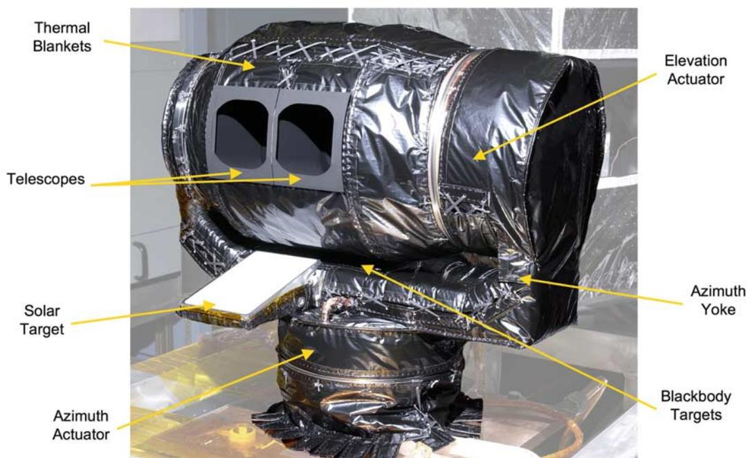
**Figure 1.** The MCS flight instrument photographed during calibration at JPL. Major elements of the instrument are identified.
